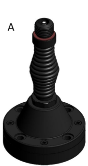
A NATO 4-hole Spring 4 x M10 or 3/8" Bolts on 114mm PCD Base diameter 140mm (5.5in) Base height 240mm (9.5in)
