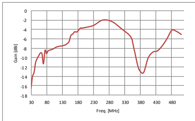
Typical gain curve mounted in centre of a 1.2m x 1.2m ground plane
