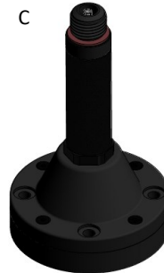
C NATO 4-hole Rigid 4 x M10 or 3/8" Bolts on 114mm PCD Base diameter 140mm (5.5in) Base height 240mm (11in)
