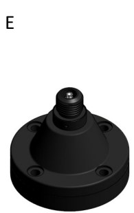
E NATO 4-hole Rigid (no spring) 4 x M10 or 3/8" Bolts on 114mm (4.5in) PCD Base diameter 140mm (5.5in)
