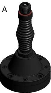
A NATO 4-hole 4 x M10 or 3/8" Bolts on 114mm (4.5in) PCD Base diameter 140mm (5.5in)
