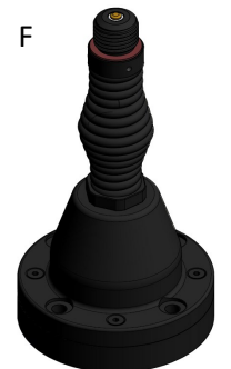
F NATO 4-hole Spring GPS Base L1 & L1/L2 GPS available 4 x M10 or 3/8" Bolts on 114mm (4.5in) PCD Base diameter 140mm (5.5in)
