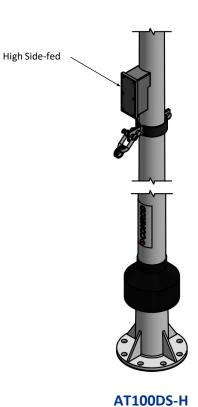
Deck mounted, side-fed (high) Uses the same side feed point as the AT100DS but it is positioned 2 metres above the base flange
