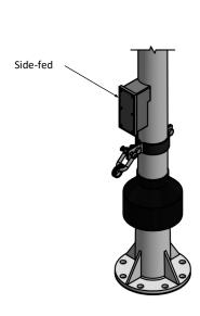
Deck mounted, side-fed Fed cable positioned 500mm above the mounting flange
