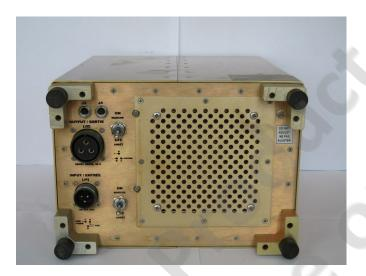
The BC1500BM TC 3S input current is power factor corrected, and is configured for optimum adaptation to weak power sources such as portable generators. The charger has signal for charger time out, (bulk stage for more than 10 hours will make the charger shut down), temperature sensor fault, battery over temperature, bulk or absorption stage, float stage and charger ON.
