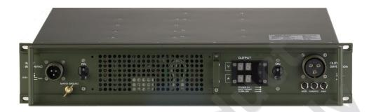
The BC 1500 RM 48V input current is power factor corrected and designed for optimum adaptation to weak power sources such as portable generators. The efficiency is very high due to the soft switching converter technology. The BC 1500 RM 48V is intended for mounting in 19" rack systems and occupies 2U (88mm) (3.5") height.
