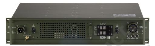
The BC 1500 RM 28V input current portable generators. The efficiency is very high due to the soft switching converter technology. The BC 1500 RM 28V is intended for mounting in 19" rack systems and occupies 2U (88mm) (3.5") height.
