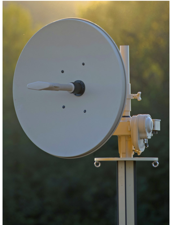
CAPAS -SR rotator with Comrod band IV antenna mounted on a Comrod TM210 electro-mechanical mast
