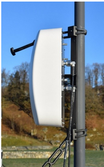
Pole mounted using rubber straps
