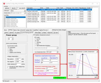
The temperature compensation characteristic is shown graphically in the bottom right corner.
