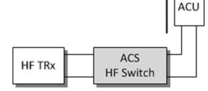
Depending on the operational profile of the submarine (surfaced, submerged, number of masts that are hoisted etc.) different frequency banks are required. These frequency banks are calibrated locally but stored in the Antenna Control System (ACS). This automatic calibration function does not require the use of a radio as a frequency synthesizer is included in the system.
