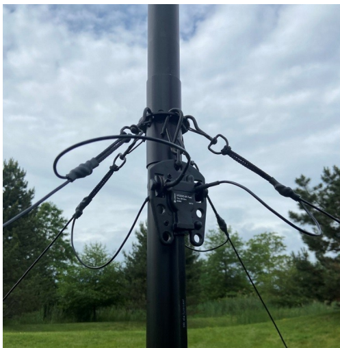
Center junction and dipole wires (shown with optional AMX85 support mast)
