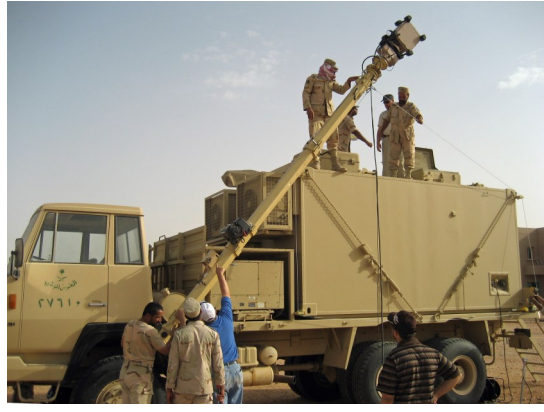
Mast weight fully supported during deployment
