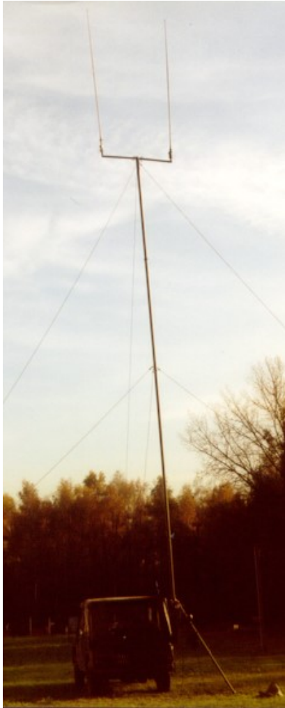
2 antennas on ULM-11/QESH mast
