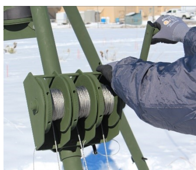
Central guying system maintains tension during deployment
