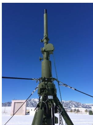
Top load attached to top mast section
