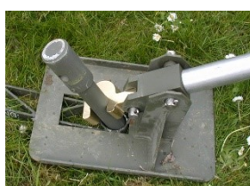
Stake remover for hard soils
