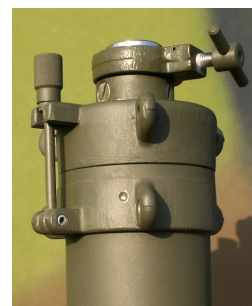
Protective top cap to secure sections in collapsed position
