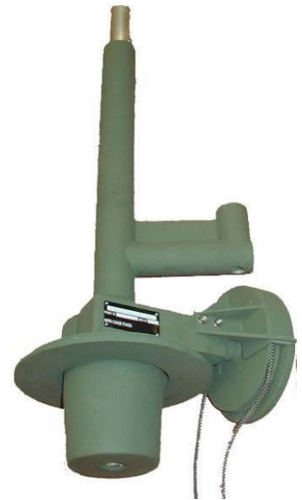
F3435-63231 Rotator - Circular flange and V-ring collar interface (fast securing system). 40mm spigot for antenna fixation. The COMROD standard lightning arrester can be directly mounted onto the integral rotator bracket.
