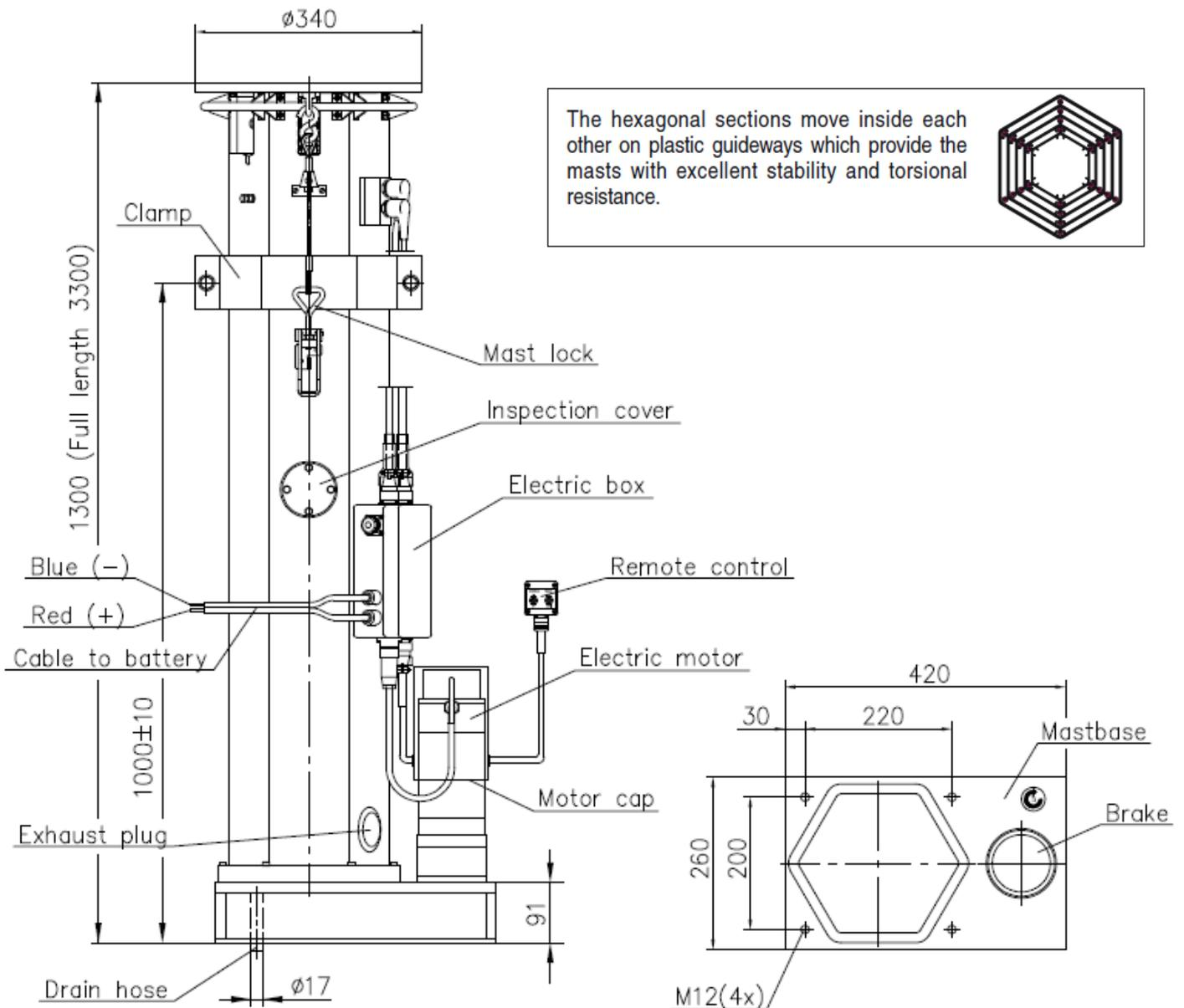
The hexagonal sections move inside each other on plastic guideways which provide the masts with excellent stability and torsional resistance.
