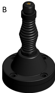
B NATO 4-hole Spring GPS 4 x M10 or 3/8" Bolts on 114mm (4.5in) PCD Base diameter 140mm (5.5in) Base height 240mm (9.5in)
