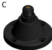
C NATO 4-hole Rigid 4 x M10 or 3/8" Bolts on 114mm (4.5in) PCD Base diameter 140mm (5.5in) Base height 100mm (4in)
