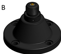
B NATO 4-hole Rigid 4 x M10 or 3/8" Bolts on 114mm PCD Base diameter 140mm (5.5in) Base height 100mm (4in)
