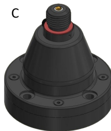
C NATO 4-hole Rigid - GPS 4 x M10 or 3/8" Bolts on 114mm PCD Base diameter 140mm (5.5in) Base height 150mm (6in)
