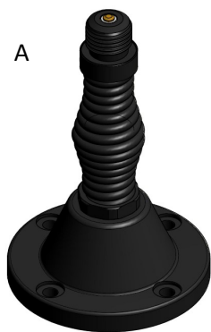
A NATO 4-hole Spring 4 x M10 or 3/8" Bolts on 114mm (4.5in) PCD Base diameter 140mm (5.5in) Base height 215mm (8.5in)
