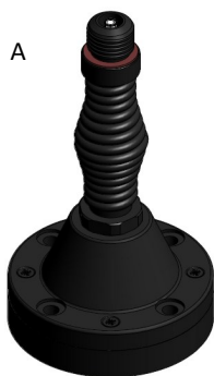
NATO 4-hole Spring 4 x M10 or 3/8" Bolts on 114mm PCD Base diameter 140mm (5.5in) Base height 240mm (9.5in)
