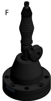
F NATO 4-hole Tilt Spring Base GPS and EMP options 4 x M10 or 3/8" Bolts on 114mm PCD Base diameter 140mm Base height 305mm
