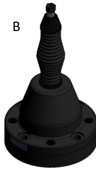
B NATO 4-hole Spring Base GPS and EMP options 4 x M10 or 3/8" Bolts on 114mm PCD Base diameter 140mm Base height 245mm
