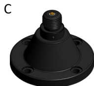
C NATO 4-hole Rigid 4 x M10 or 3/8" Bolts on 114mm PCD Base diameter 140mm (5.5in) Base height 100mm (4in)
