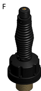
F NATO 50mm Thread GPS with Spring Base diameter 95mm (3.7in) Base height 230mm (9in)
