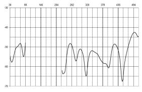
Typical isolation between VHF/UHF ports
