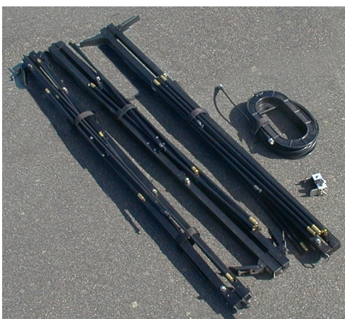
Antenna shown collapsed for transportation
