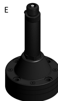
E NATO 4-hole Rigid (no spring) 4 x M10 or 3/8" Bolts on 114mm (4.5in) PCD Base diameter 140mm (5.5in)
