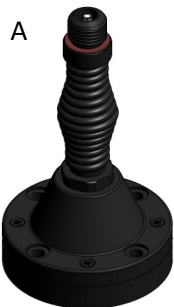
A NATO 4-hole 4 x M10 or 3/8" Bolts on 114mm (4.5in) PCD Base diameter 140mm (5.5in)
