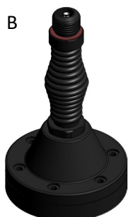
B NATO 6-hole 6 x M6 or 1/4" Bolts on 111mm (4.37in) PCD Base diameter 140mm (5.5in)
